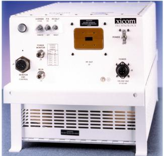
The XTD-750 is a compact, self-contained, antenna mountable power amplifier designed for low cost installation and long life. The XTD-750 design eliminates the need for an amplifier shelter as well as a long waveguide run between the amplifier and antenna feed horn. RF filters, cooling, and monitoring & control (M&C) systems are all self-contained within the High Power Amplifier (HPA). These features provide high reliability, low maintenance costs, and low replacement costs.
